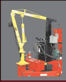
Hoist w/ Manual or 12-Volt Electric Winch
