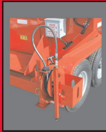
Spray System Hose Reel
