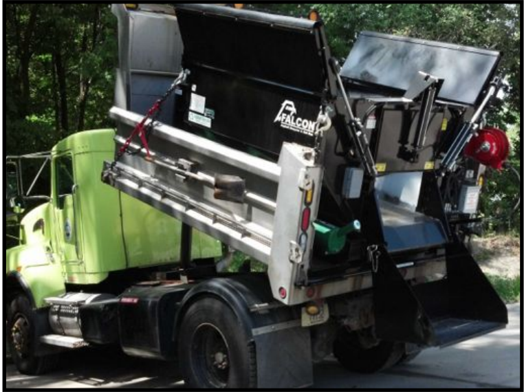
5-Ton Dual Burner Slip-in with Heated Tack Tank, Spray System and Other Options
