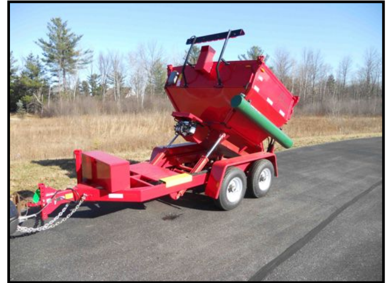
2-Ton Dump Box with Arrow Stick, 24-Hour Timer and Hydraulic Doors
